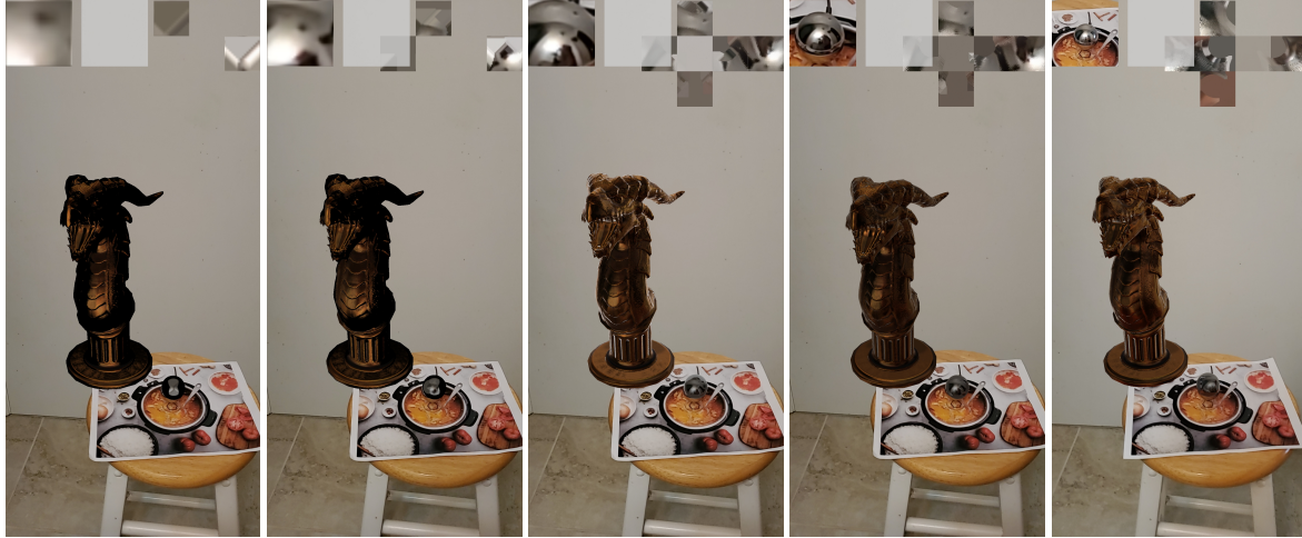
Figure 2. From left to right are the results of using GLEAM with resolutions of 16 pixels, 32 pixels, 64 pixels, 128 pixels, and 256 pixels. The cubemap that is used for each resolution is shown in the top right hand corner of each image. In the left hand corner is the image of the probe that is being used to generate the cubemap.
